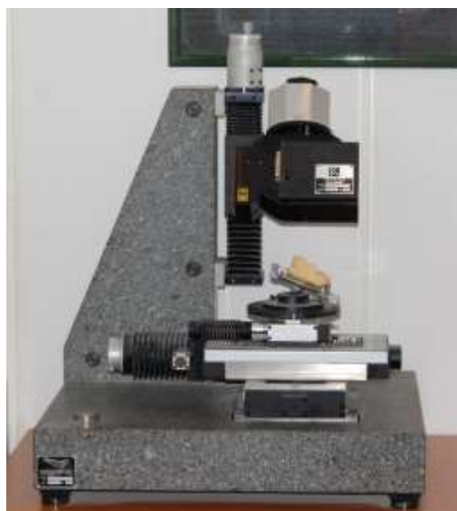
Figure 2: CICERO®: First laser-line laboratory scanner [12].
